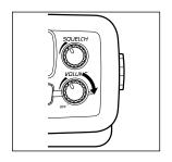
**Note:** You must select a channel which is not in use before setting the **SQUELCH** control on your radio.
